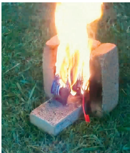
Figure 1: Burning lithium-ion battery
