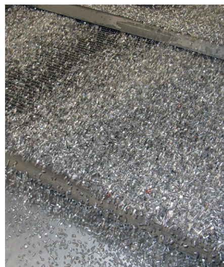
Figure 3: Aluminium granulate from cable recycling
