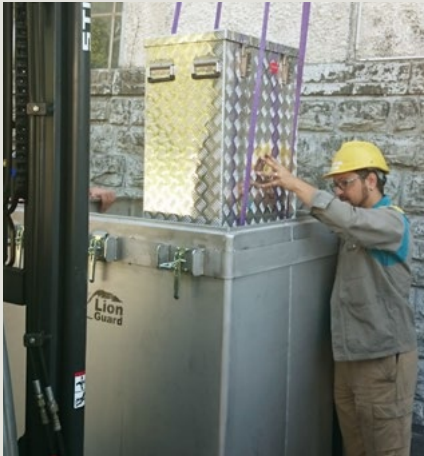
Figure 3: The UN-approved collection containers are lifted by harness into and out of the transportation containers.
